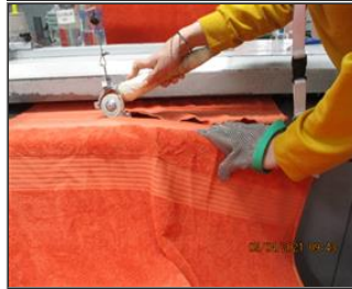
Photo of the personal protection equipments (if applicable) ppe in cutting section.JPG
